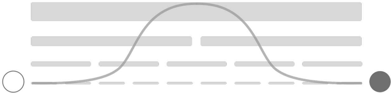
Fig. 4 - A packet traverses zones of various sizes from the origin node to the destination node
